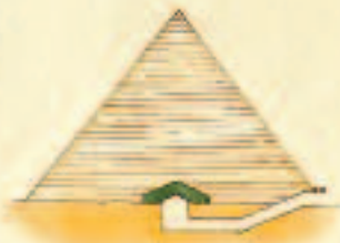
This is a cross-section through the pyramid as it will look when complete. The entrance is at ground level. The positioning of the blocks that make up the roof of the burial chamber form a peaked shape. This is designed to support the enormous weight of pyramid blocks above it.
