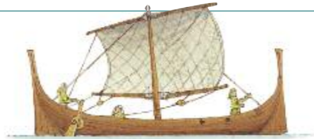
About 1000 years ago, the Vikings, who lived in northern Europe, started to explore new lands. Their ships were called knorrs (above). Each had a hull (body of vessel) made of overlapping or "clinkered" planks.
